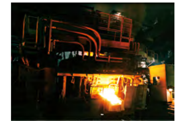
Upgraded 50 ton electric furnace
