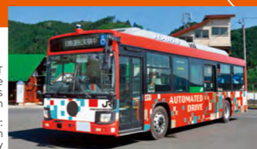
Large autonomous BRT bus equipped with the GMP5 autonomous driving support system Photograph provided by: East Japan Railway Company
