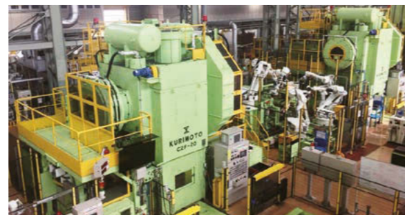
▲ Newly adopted forging machine used to manufacture ring gears
