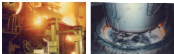
80-ton electric arc furnace (left), Vacuum degassing unit (right)
